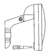
The Corner Patch 7.5 dBi with coaxial cable. The DirectLink Corner Patch antenna mounts on walls near the ceiling or on rooftops. The
