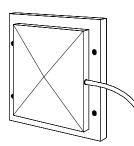
The Panel antenna mounts on walls near the ceiling or on rooftops. The antenna will, in this usage clearly will be more than 20 cm from the user
