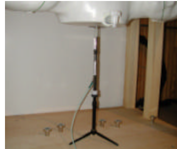
Figure 12.1 Dipole Validation Test Setup
