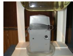
Figure 14.3 Body SAR Test Setup
