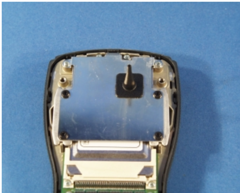
Antenna Photograph Installed
