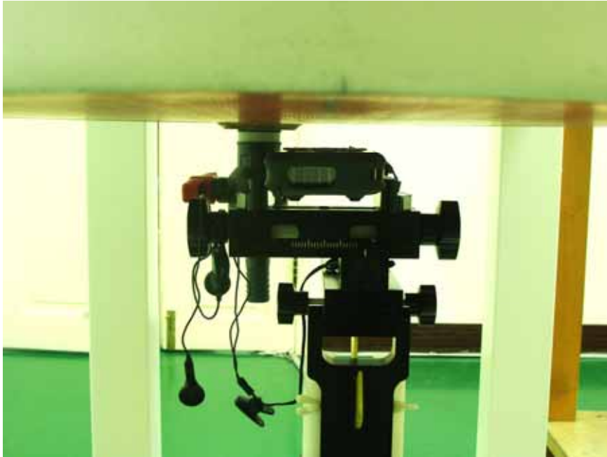
Face of the DUT with Battery 1 - with Phantom 1.5 cm Gap
