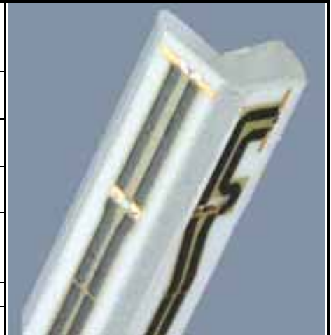
Fig. 5.2 E-field Free-space Probe
