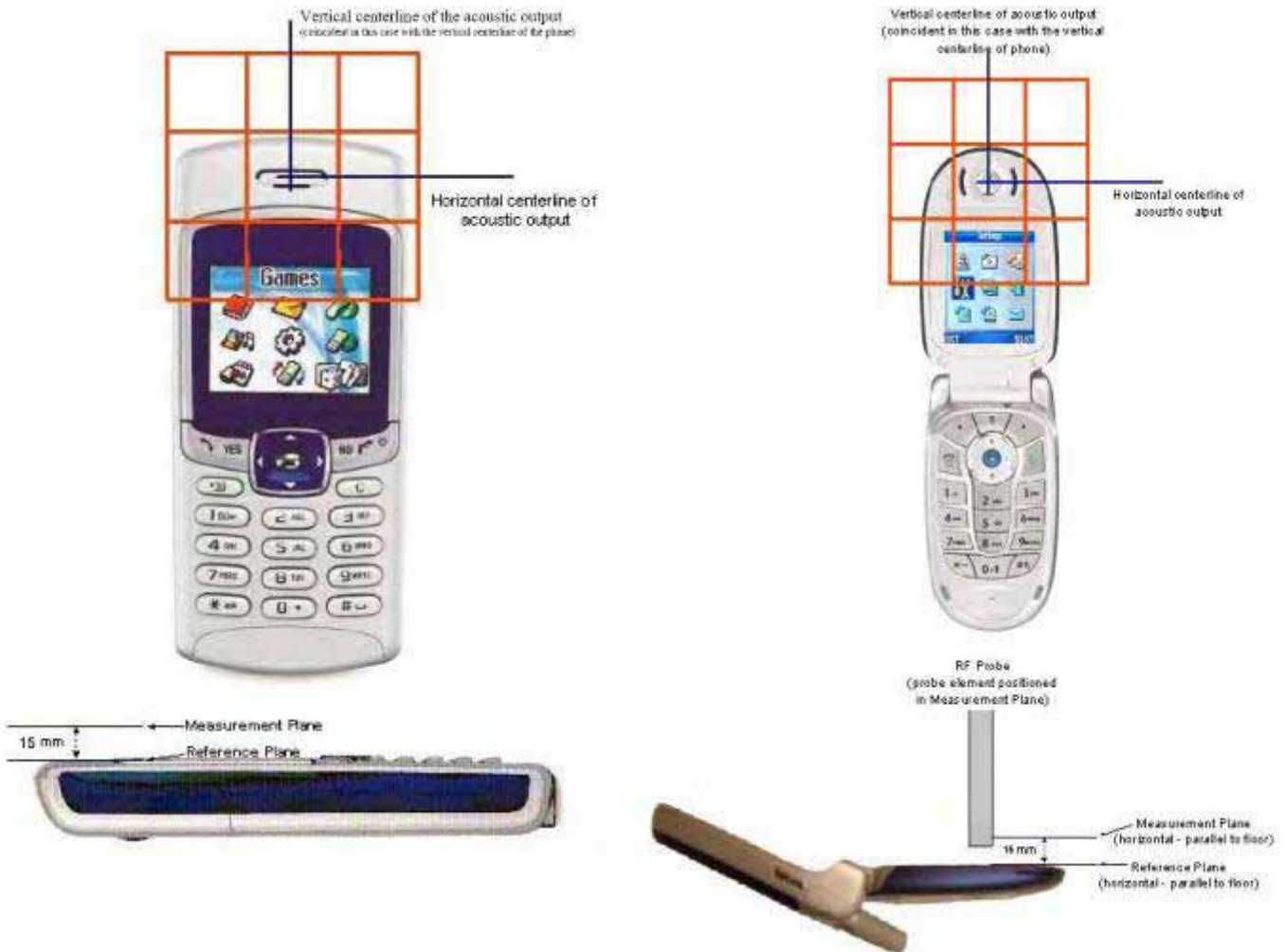
Figure 9.1: A typical DUT reference and plane for HAC measurements
