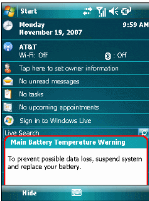
Figure 2-9 Main Battery Temperature Warning Dialog Box
