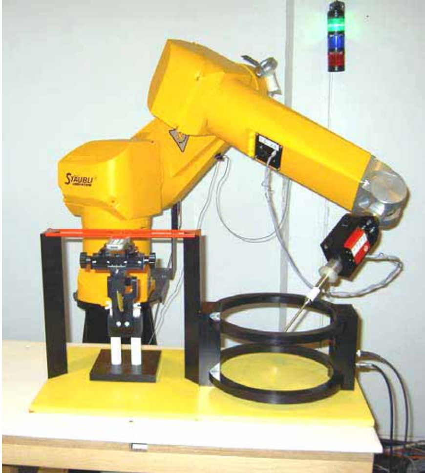
Figure 5.1: T-Coil setup with HAC Test Arch and AMCC
