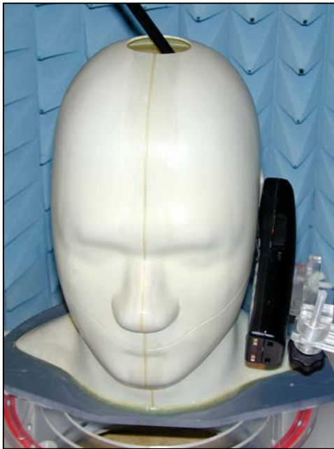
Figure 27. Positional photograph of the NetVision® Phone Handset in the Left-hand Cheek Position
