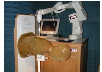
Fig. 1 SAR Test Setup
