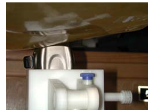
Fig. 10 Hand SAR Test Setup
