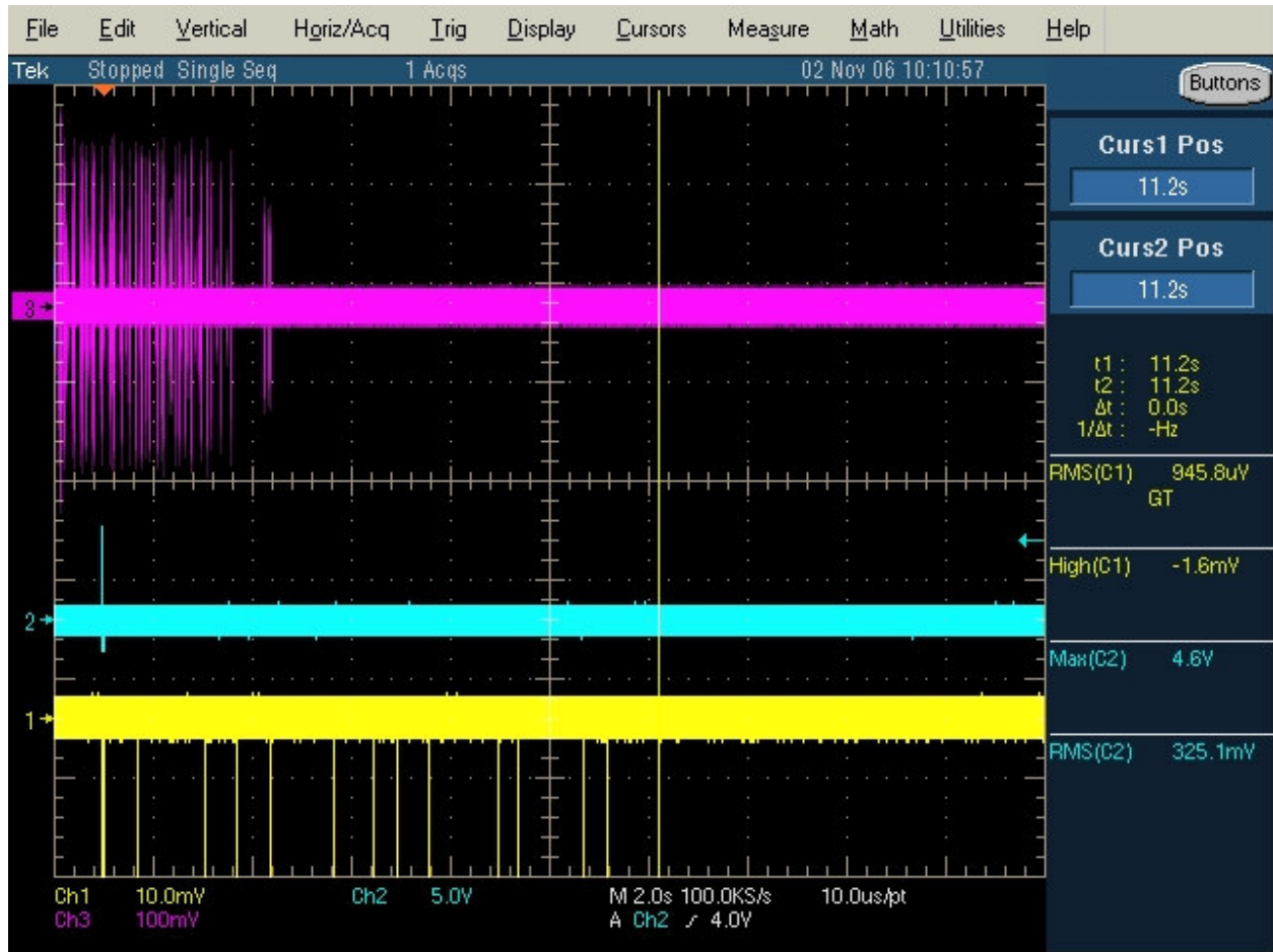
Radar Type 5 FCC Closing and Moving time plot (Channel Moved before radar pulse completed)
