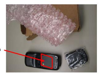
The other type of shipping container has one unit wrapped in bubblewrap with a separately packaged battery.
