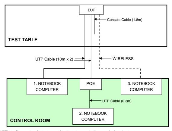
**NOTE:** 1. Support unit 1~3 were kept in the control room during the test.
