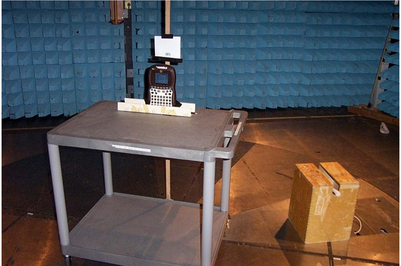
Spurious Radiated Emissions Set Up Photograph
