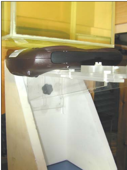
Figure 18. Positional photograph of the Symbol 4121CDMA Handheld Data Terminal in Front Touch Position
