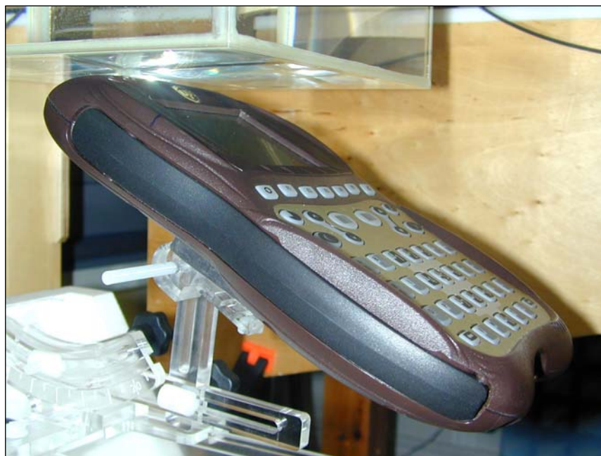
Figure 20. Positional photograph of the Symbol 4121CDMA Handheld Data Terminal in Front Tilt Test Position
