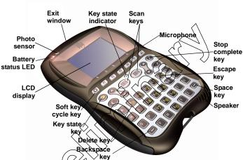
Note: The battery status LED lights only when the battery is charging in the DIAD IV Depot Charger. When the terminal is not charging, this LED is application dependent.
