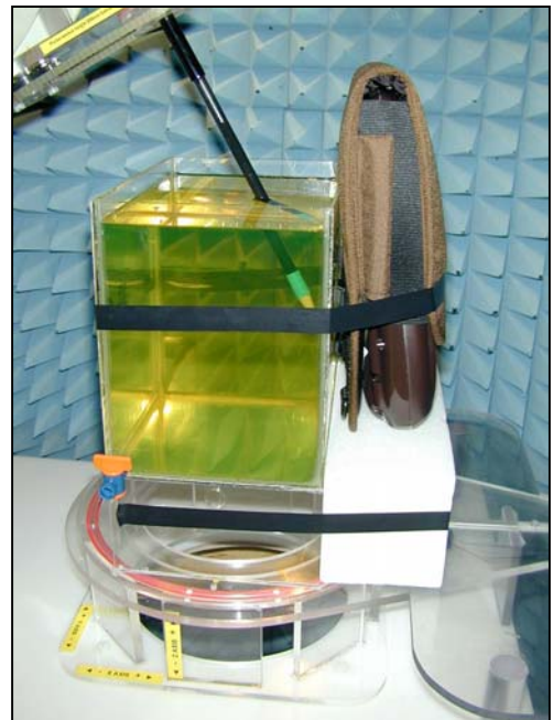
Figure 39. Positional photograph 4111-GPRS Touch Position Rear Facing inside wallet
