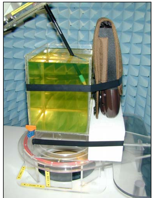
Figure 36. Positional photograph 4111-CDMA Touch Position Rear Facing inside wallet
