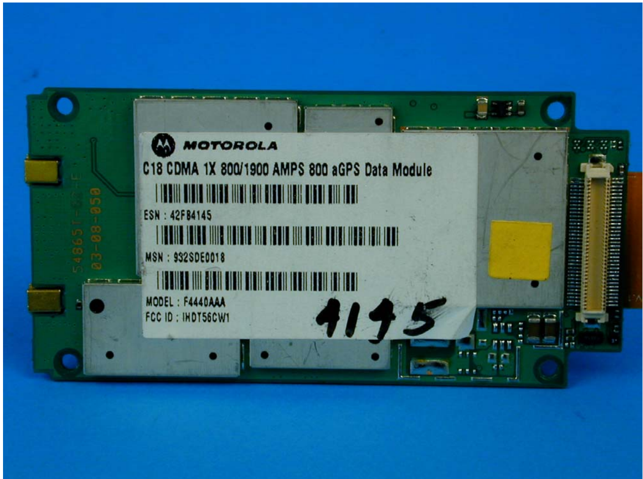
Photograph 11 4111-CDMA Front View of C18 CDMA Module
