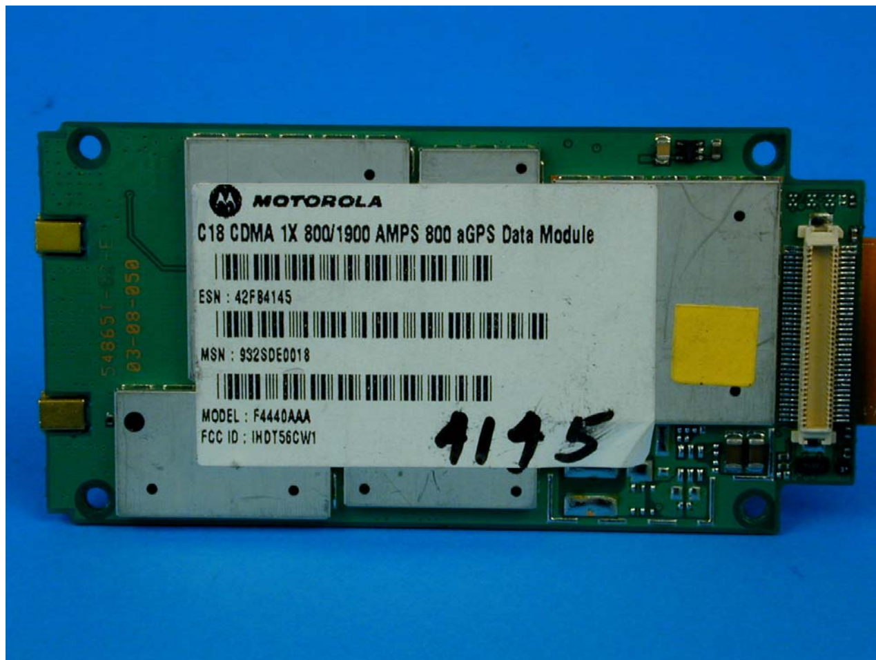
Photograph 11 4111-CDMA Front View of C18 CDMA Module
