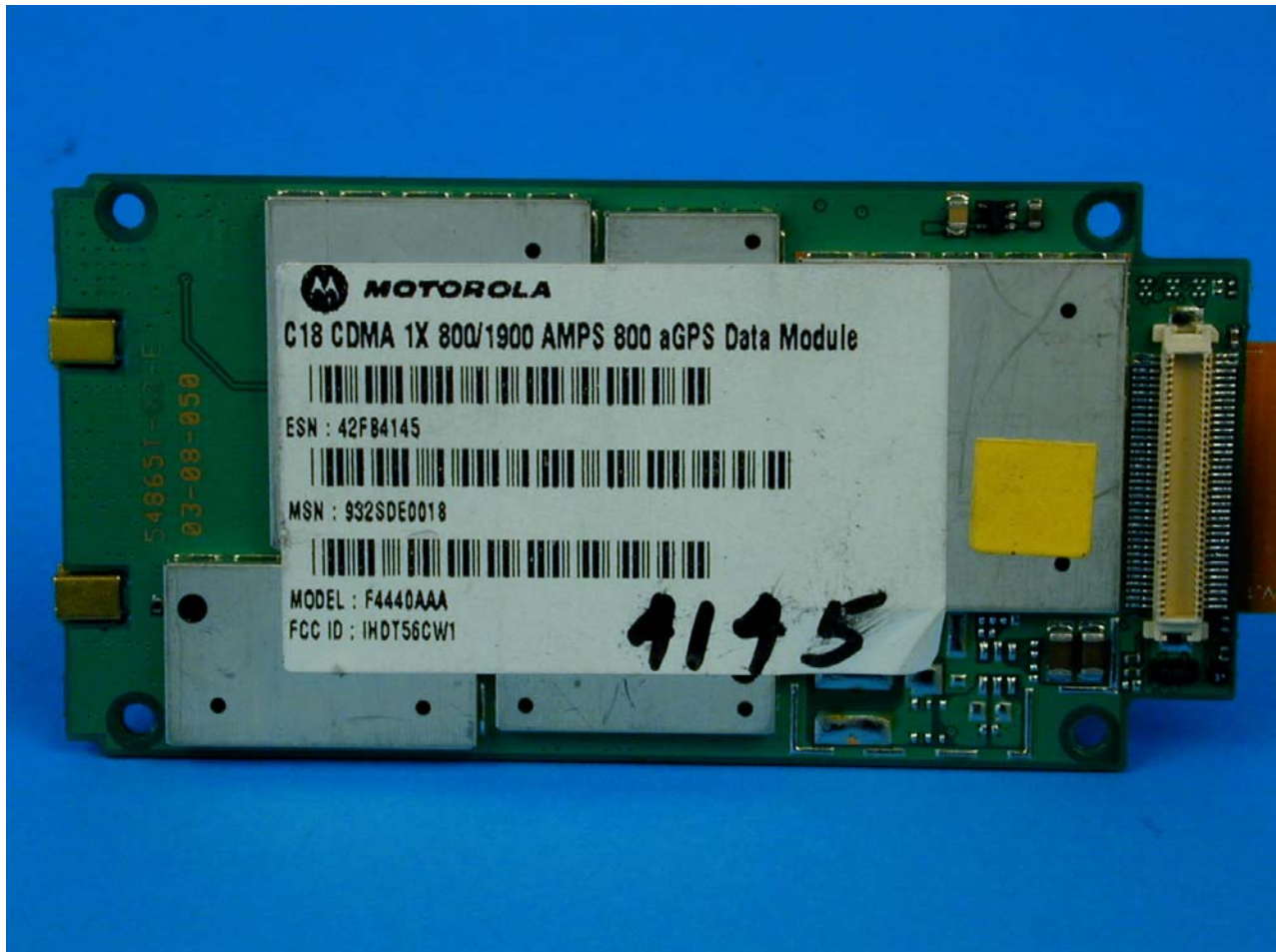
Photograph 11 4111-CDMA Front View of C18 CDMA Module
