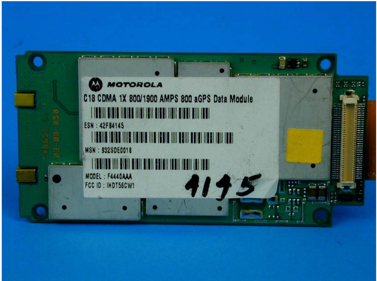
Photograph 11 4111-CDMA Front View of C18 CDMA Module
