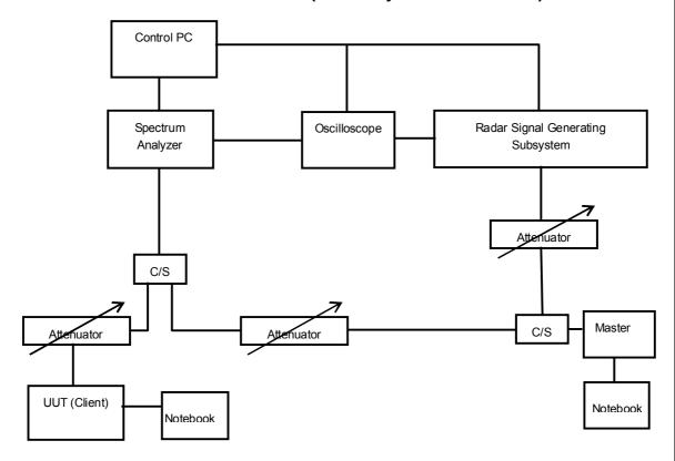
The UUT is a U-NII Device operating in Client mode with radar detection. The radar test signals are injected into the Master Device.
