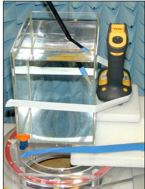
Figure 25. Positional photograph of the LS3478 RHS facing to Phantom side
