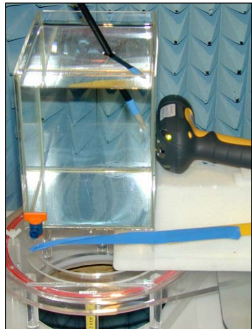
Figure 27. Positional photograph of the LS3478 Top facing to Phantom side
