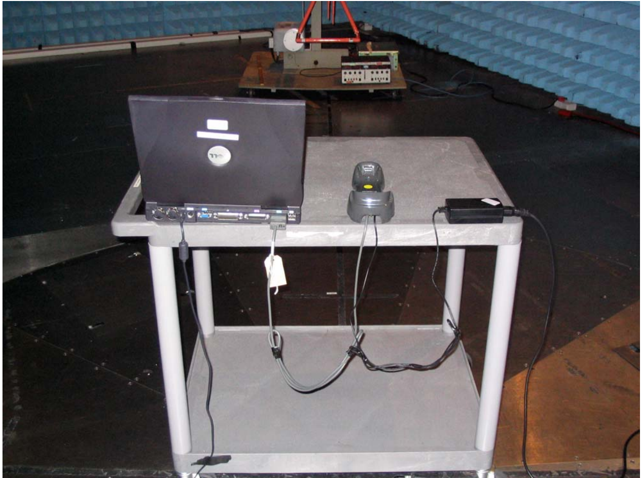
Spurious Radiated Emissions Set Up Photograph
