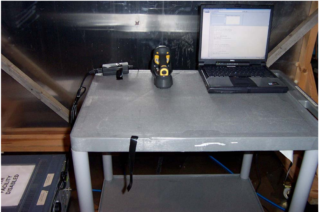
Conducted Emissions Set Up Photograph
