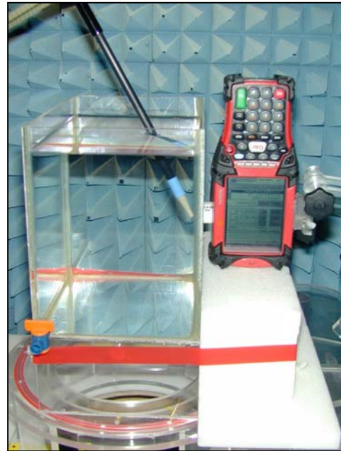
Figure 26. Positional photograph of the MC9060 Right-hand side at 1.0cm from Phantom side
