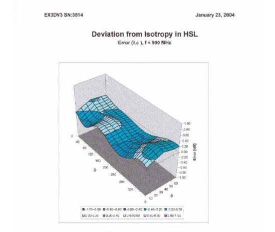
Spherical Isotropy Error < ± 0.4 dB
