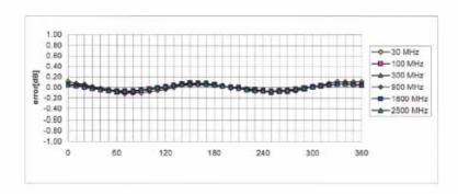
Axial Isotropy Error < ± 0.2 dB
