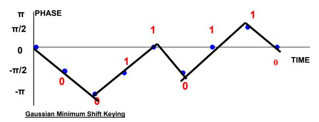
MSK has high sidebands relative to the main lobes in the frequency domain - this can lead to interference with adjacent signals.
