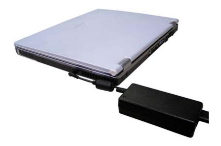
While the AC adapter works with electrical outlets worldwide, power connectors and power strips vary from country to country. Ensure you use compatible cable or correctly connect the cable to the power strip or electrical outlet. Failure to do so may cause fire or damage to equipment.
