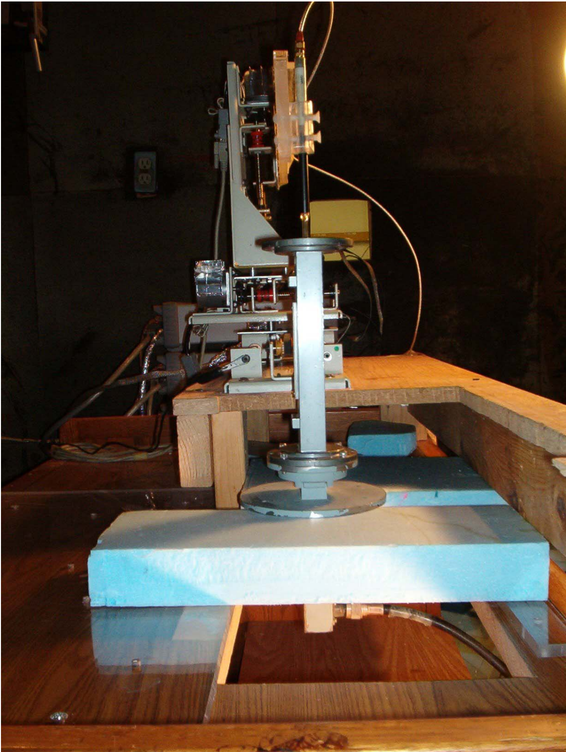
Fig. 7b. Photograph of the waveguide setup showing also the coax to waveguide coupler at the bottom used to feed power to the vertical waveguide containing the tissue-simulant fluid.
