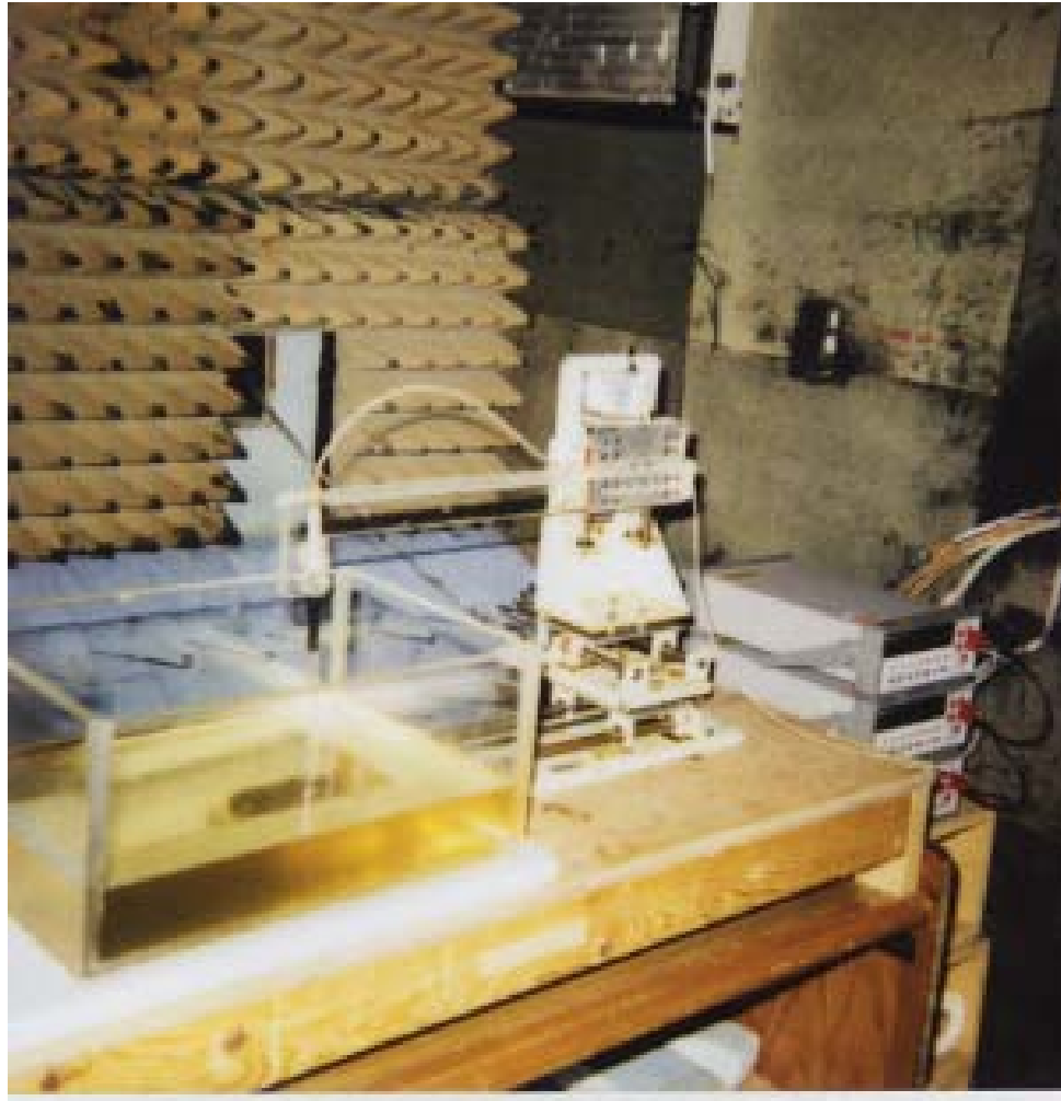
Fig. 5. Photograph of the three-dimensional stepper-motor-controlled SAR measurement system using a planar phantom (see Figs. 3 and 4 for a detailed examination of the placement of the Model BCL50 Notebook Computer with Askey Model WLL220 802.11a Wireless Antennas relative to this phantom).
