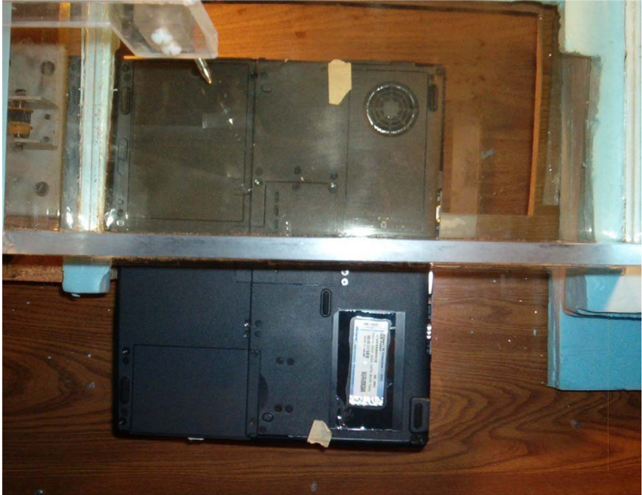
a. The right half of the PC with antenna "A" pressed against the planar phantom.
