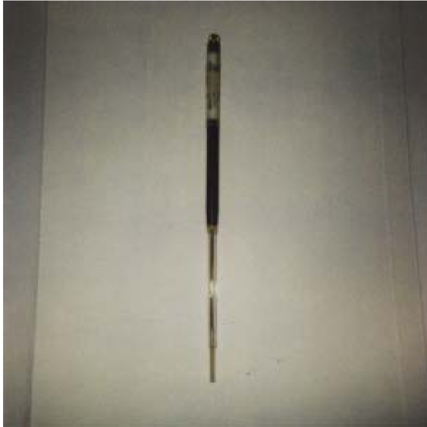
Fig. 8. Photograph of the Narda Model 8021 Broadband Electric Field Probe used for SAR measurements.
