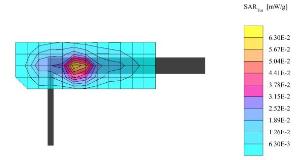
Separation distance: 0mm (EUT Tip to Phantom)
