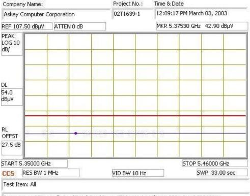
Description: 802.11 a/b Dual Band Card Bus in IBM Laptop, M/N WLC221-D4, BCP3483U Transmit at 5.32 GHz, ATR=15, Vertical Aerage.
