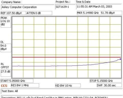
Description: 802.11 a/b Dual Band Card Bus in IBM Laptop, M/N WLC221-D4, BCP3483U Transmit at 5.18 GHz, ATR=15, Average.
