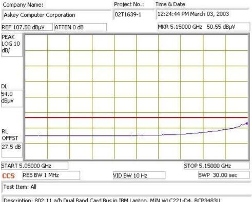
Description: 802.11 a/b Dual Band Card Bus in IBM Laptop, M/N WLC221-D4, BCP3483U Transmit at 5.18 GHz, ATR=15, HORIZONTAL Average Low area
