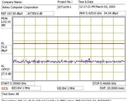
Description: 802.11 a/b Dual Band Card Bus in IBM Laptop, M/N WLC221-D4, BCP3483U Transmit at 5.32 GHz, ATR=15, HORIZONTAL Peak High area
