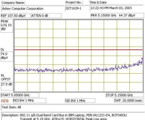
Transmit at 5.18 GHz, ATR=15, HORIZONTAL Peak Low area
