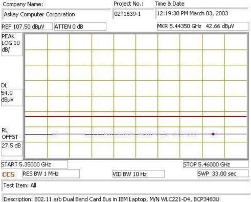
Description: 802.11 a/b Dual Band Card Bus in IBM Laptop, M/N WLC221-D4, BCP3483U Transmit at 5.32 GHz, ATR=15, HORIZONTAL Average High area
