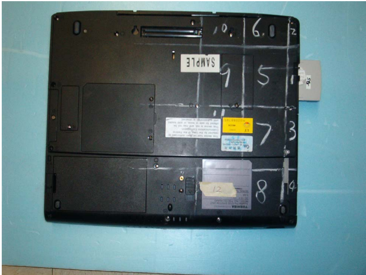
Fig. A. A photograph of the bottom side of the Toshiba Satellite Pro 6100 Laptop Computer with the Askey Corporation Model WLC221-D4 Cardbus Card inserted in it. Marked here are the various regions 1-12 each of dimension 5.6 \times 8.0 cm that have been scanned for SAR distributions with a coarse scan resolution of 0.8 cm (8 mm).
