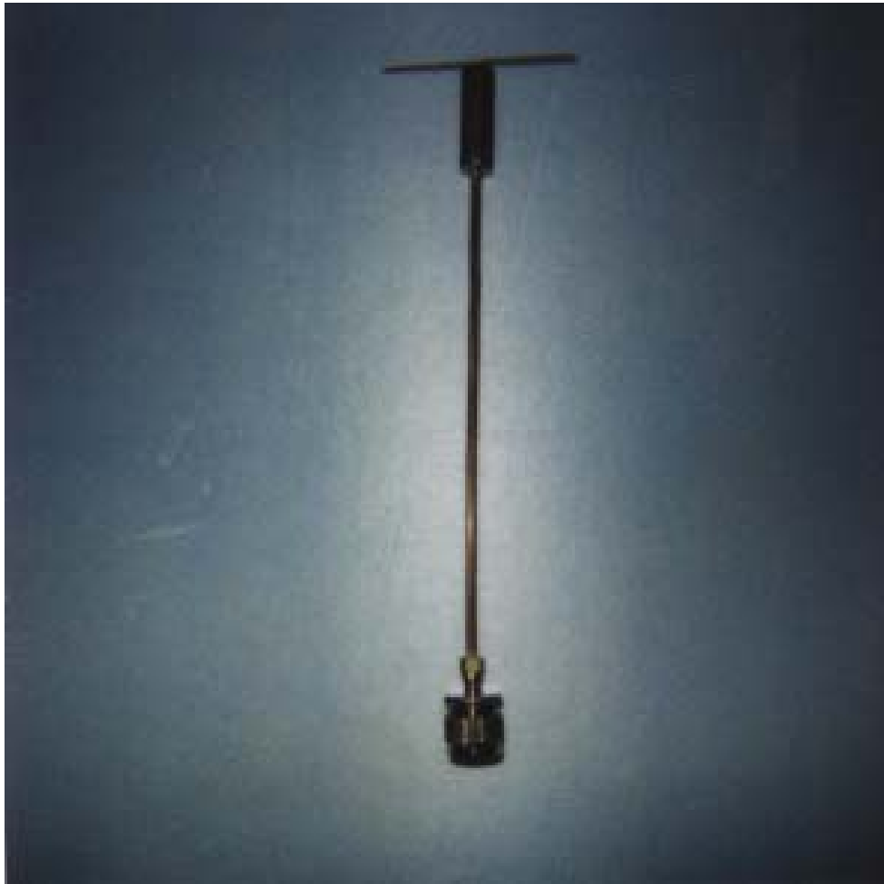
Fig. 9. Photograph of the half-wave dipole at 1900 MHz used for system verification.
