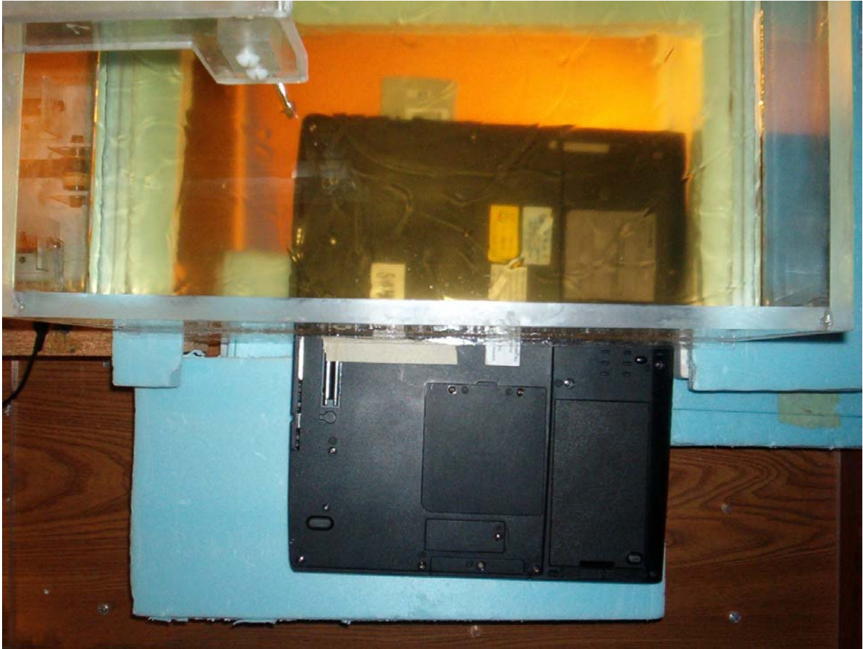
Fig. 5. Photograph of the Askey Corporation 802.11 a/b Cardbus Card inserted into a Toshiba laptop computer with its bottom pressed against the bottom of the planar tissue-simulant phantom to simulate "above-lap" placement of the wireless PC. A Styrofoam block is used under the base to prevent bending of the 2 mm thin base of the phantom.
