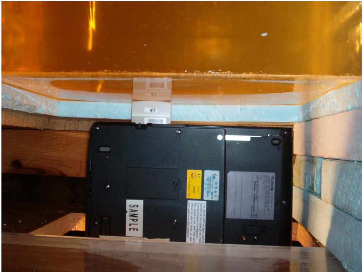
Fig. 6. Photograph of the Askey Corporation 802.11 a/b Cardbus Card inserted into a Toshiba portable computer (as in Fig. 1) placed with the card edge at 90^\circ and separated from the bottom of the phantom by 0 cm for "end-on" testing of SAR. As in Fig. 5, here too, a Styrofoam block is used under the base to prevent bending of the 2 mm thin base of the phantom.
