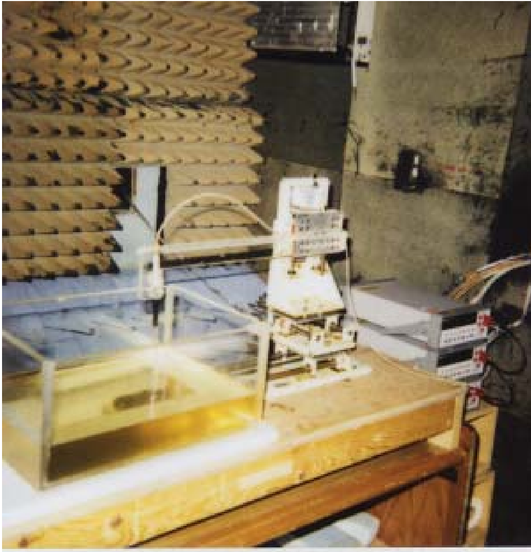
Fig. 3. Photograph of the three-dimensional stepper-motor-controlled SAR measurement system using a planar phantom (see Figs. 5, 6 for a detailed examination of the placement of Askey Corporation 802.11 a/b Cardbus Card relative to this phantom).
