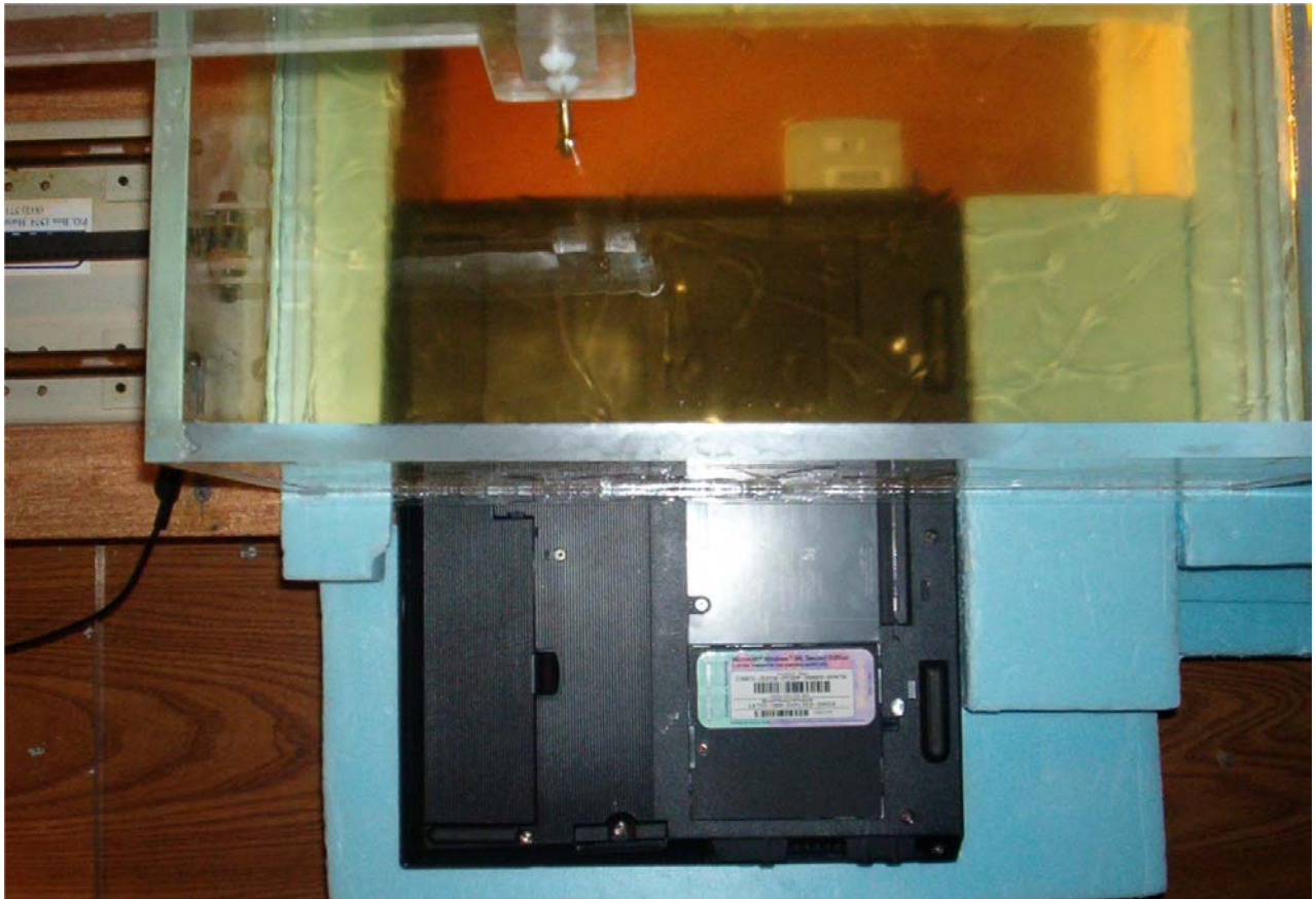
Fig. C. Photograph of the Askey Corporation 802.11 a/b Cardbus Card inserted into the IBM Model 2628 laptop computer with the PC bottom pressed against the bottom of the planar tissue-simulant phantom to simulate "above-lap" placement of the wireless PC. (This is a redone version of Fig. 5 of the SAR Test Report submitted November 21, 2002).
