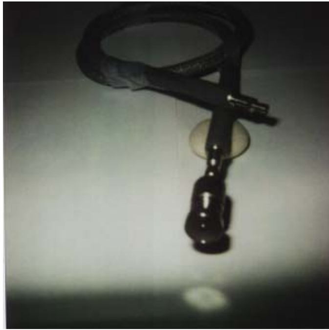
Fig. 10. Photograph of the Hewlett Packard Model 85070B Dielectric Probe. This is an open-circuited coaxial line probe.
