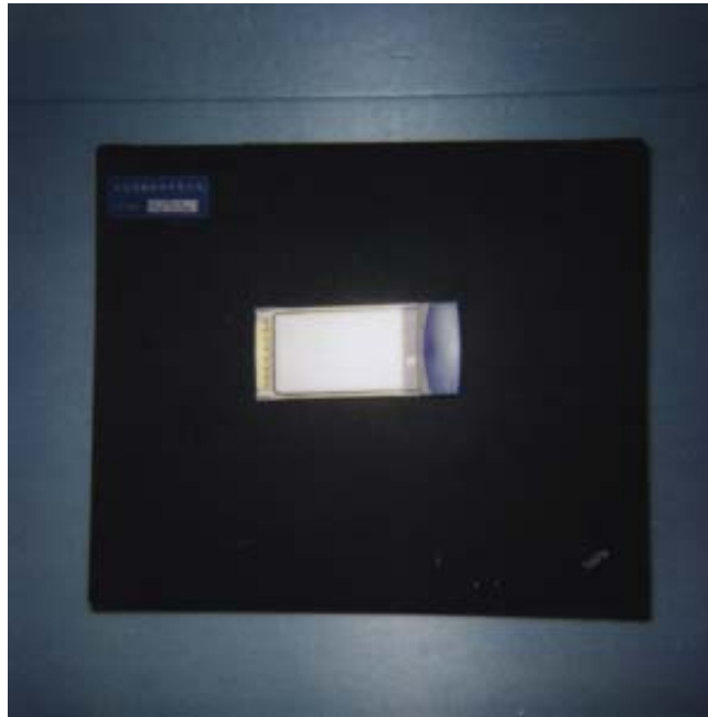
Fig. 2. A picture of the Askey Corporation 802.11 a/b Cardbus Card placed on the laptop computer.
