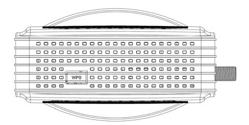
$\bigcirc$  WPS – Indicates the status of the WPS (Wi-Fi Protected Setup<sup>TM</sup>) functionality.
