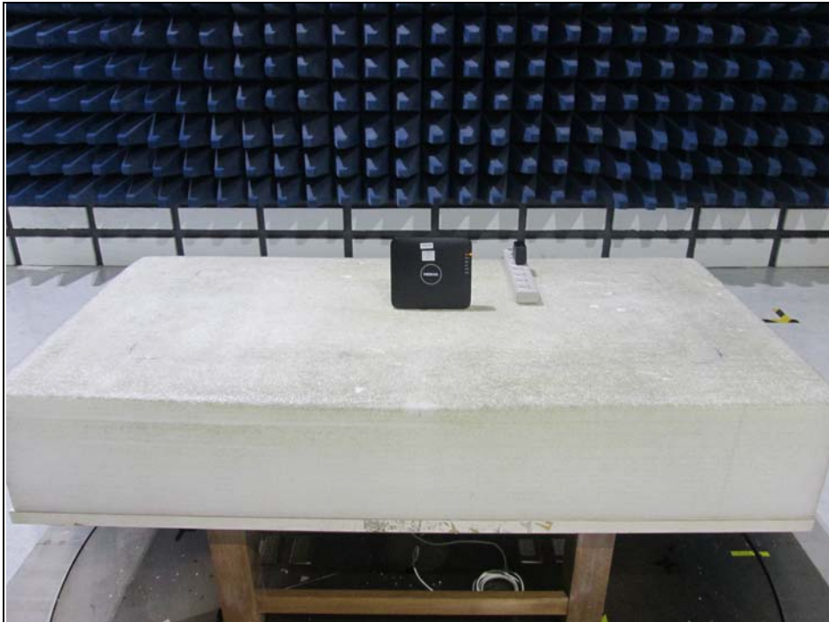
Radiated Emissions below 1 GHz Test
