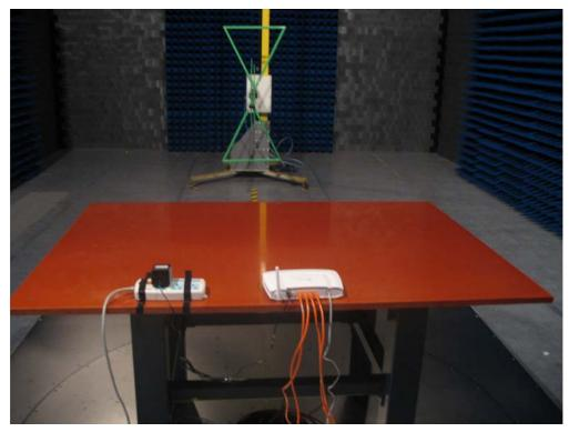
Test Mode: Mode2: Transmitter 802.11g
