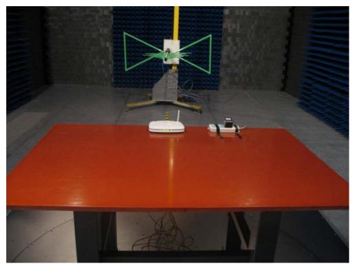
Test Mode: Mode2: Transmitter 802.11g
