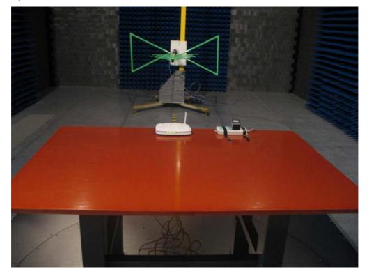
Test Mode: Mode1: Transmitter 802.11b
