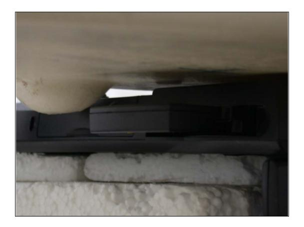
EUT to the phantom distance 11mm
