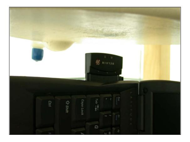
EUT to the phantom distance 15mm
