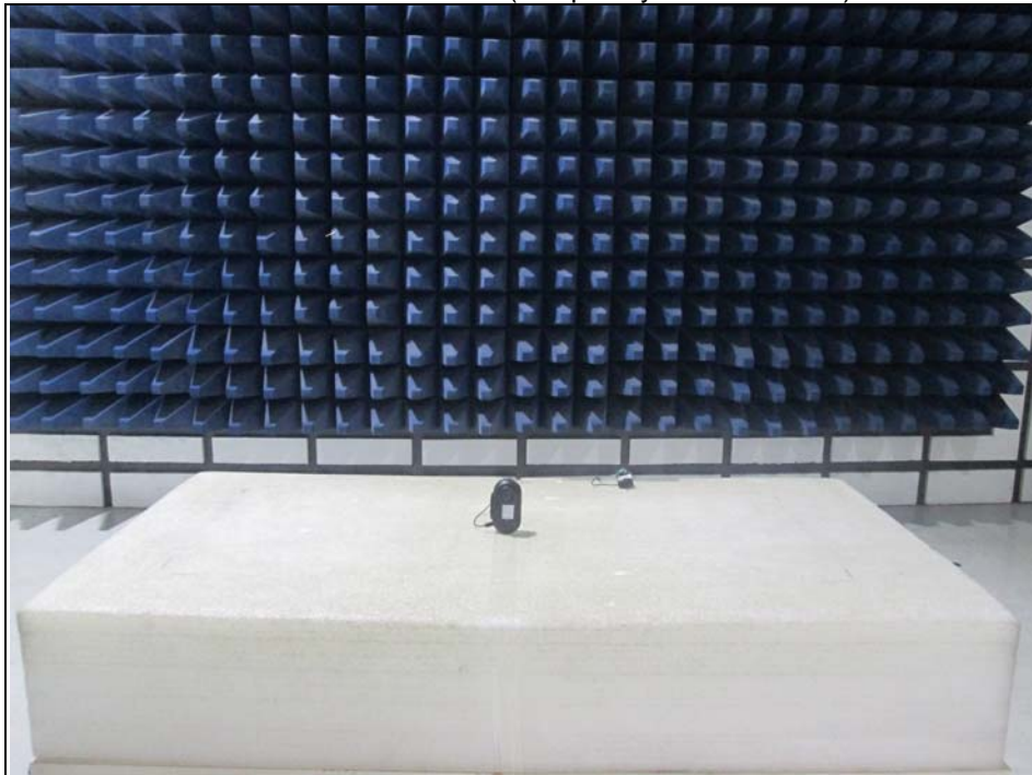
Radiated Emission Test (Frequency above 30MHz)
