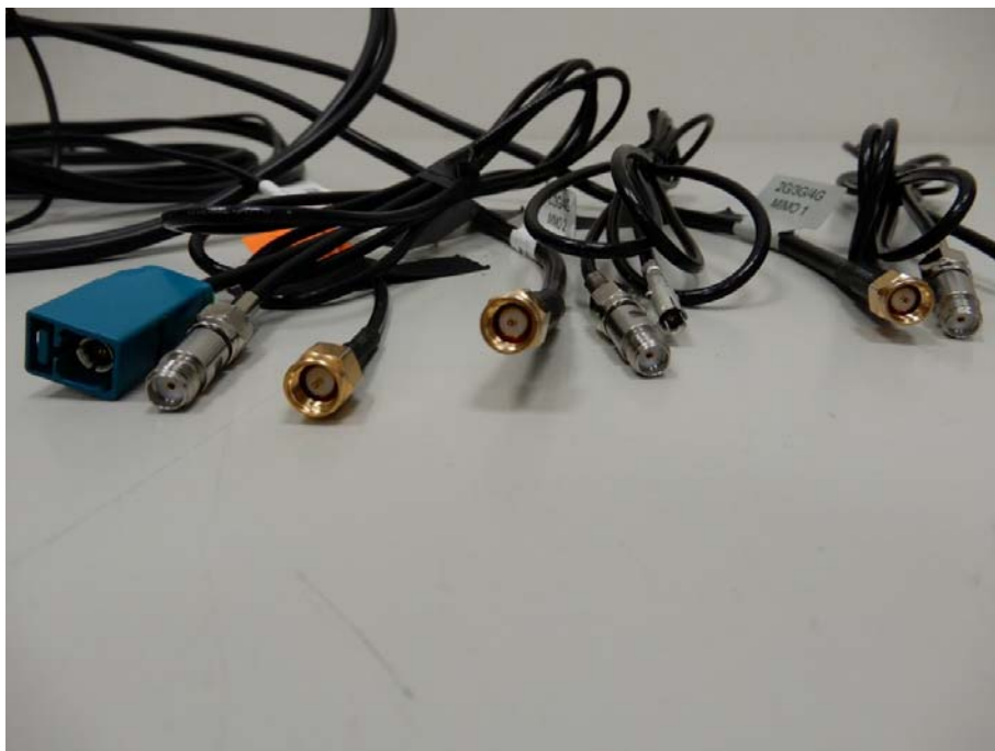
(24) EUT Photo_ LTE-4G/3G/2G MIMO Antenna Cable Zoom-In (taogles)
