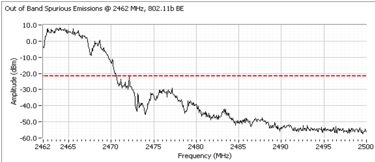
Out of Band Spurious Emissions @ 2462 MHz, 802.11b
