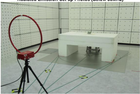
Radiated Emission Set up Photos (Below 1GHz)
