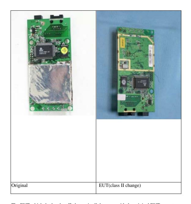
The EUT which do the class II change is all the same with the original EUT except the shielding of backside. We re test it again and have new test report for you.
