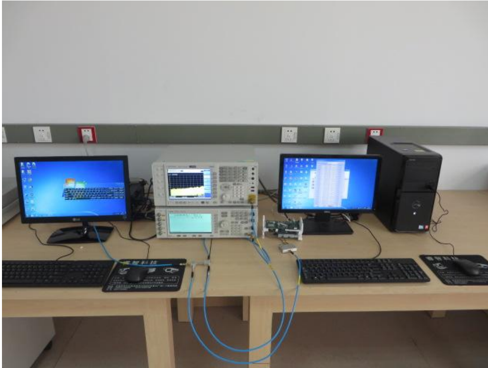
Description: Dynamic Frequency Selection Test Setup Photo
