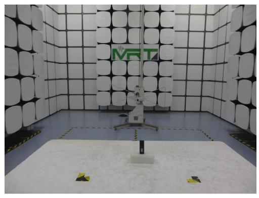
Description: Radiated Spurious Emission Test Setup for 1GHz ~ 18GHz
